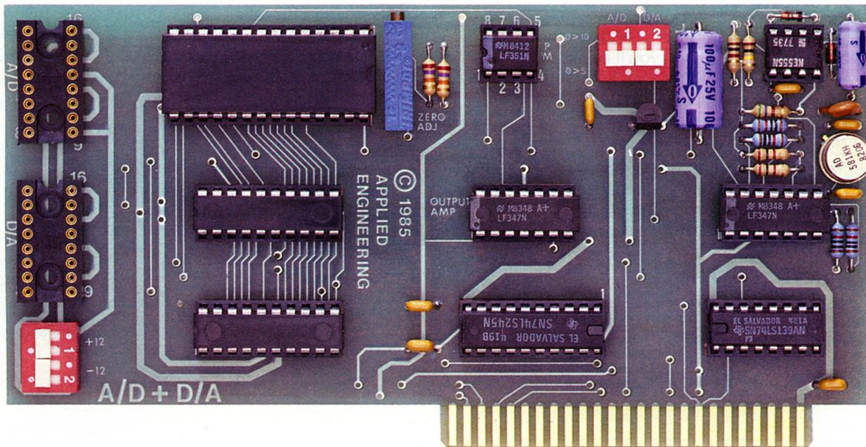
Commercial, industrial, and scientific data acquisition and control functions are now practical with Applied Engineering's A/D + D/A card.
