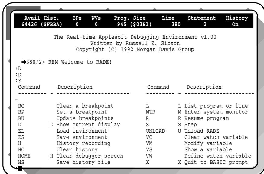
Commands you can enter in the command line are listed under the Command heading.
