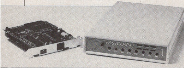
The Fastcomm Modem 2496 series can transmit data at 300, 1200, 2400, and 9600 bps and is available in internal, external, and rack-mount versions.
