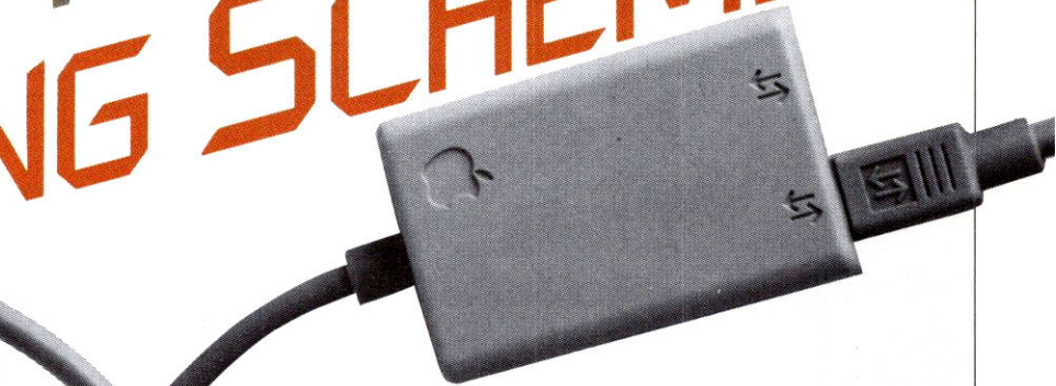
Figure 1: A LocalTalk connector, showing the connection box and drop cable. The drop cable connects to the IIe or IIgs.
