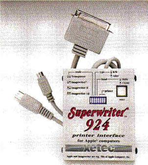
A flexible printer interface for the Apple GS, C+, and C. Emulates the Imagewriter I and II on popular 9-wire printers and the Imagewriter LQ on 24-wire printers. Cables included.
