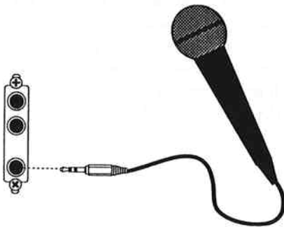
Connecting a microphone to the SoundMeister using a 3.5mm plug.
