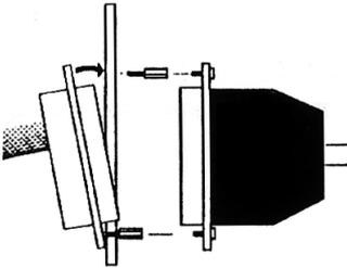
3. Loosen the bottom screw on the nut plate (but do not remove it). Remove the top screw, tilt the nut plate and slide it into the tab hole. Tilt the nut plate back to the vertical position, replace the top screw, and retighten the bottom screw.
