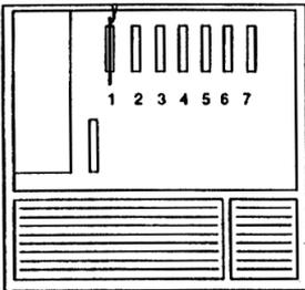
4. Although the Super-Comm card will work in any slot, slot 1 is recommended if a printer is being used, and slot 2 if a modem is being used. (For other devices, use the slot recommended in the manual that came with that device.) Install by firmly seating the card in its slot, being careful not to rock it from side to side.
